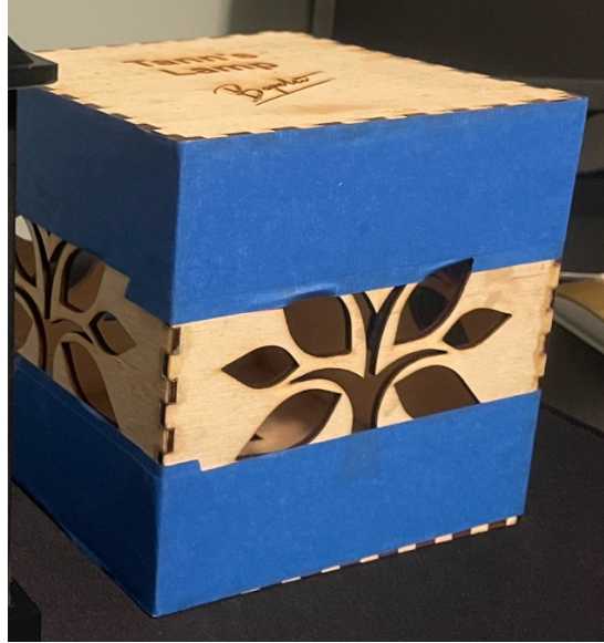
Laser Cutting Lamp Box After Assembly using glue and tape
